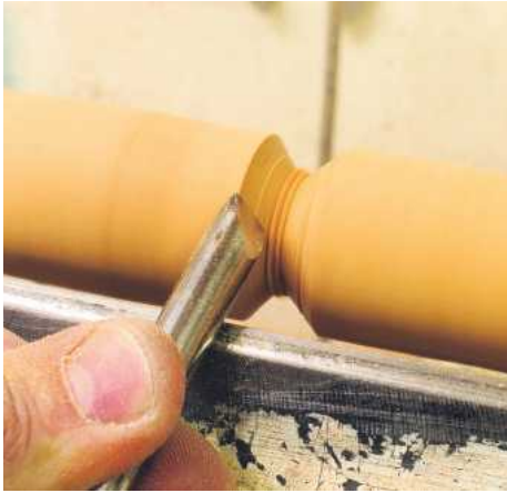
▲ Pic.19 The 10mm skew is used for all the V cuts as it achieves really sharp deep grooves. Be careful about thinning the work down too much too quickly
